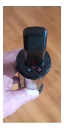
The switch on the microphone body will mute the microphone.
